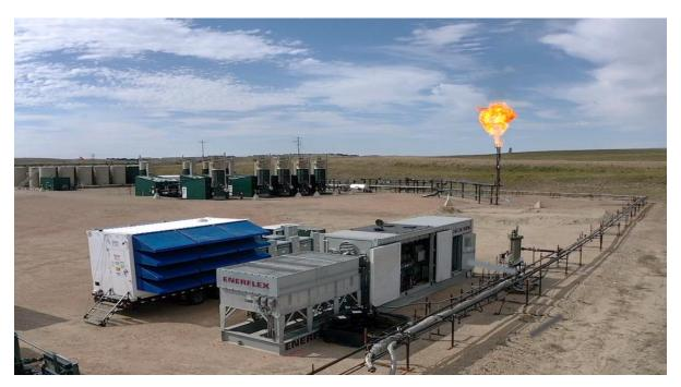
To combat these issues the Company has moved to immersion cooled units. Immersion units consist of dialectic filled tanks that recirculate cooled fluid to cool the servers. These tanks are housed in standard 40' shipping containers. Digital Stream Energy will be deploying two-1mW immersion cooling Portable Data Centers in April 2022 for Hess. During operation the units are sealed to remove any impact from fluctuating temperatures or precipitation.
