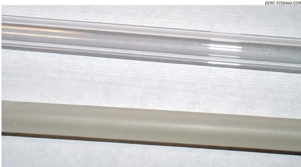
Figure 2. Quartz elements prior to mounting and cross-sectioning. The top electrode is the “blank,” the bottom element is the “spent.”
