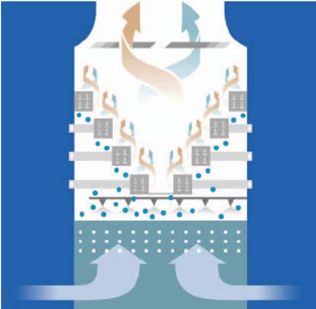
Figure 3. Schematic of SPX ClearSky system with the Air2Air mounted above the cooling tower packing.
