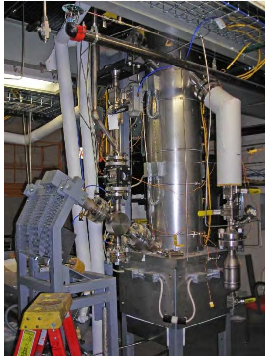
Figure B-3. Photograph of the lower section of high-pressure FBG. Visible at left is the feed auger angled downward into the bed.
