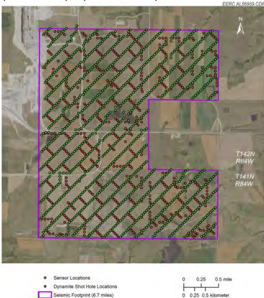
Figure 3. Survey area, sensor locations and dynamite shot hole locations
