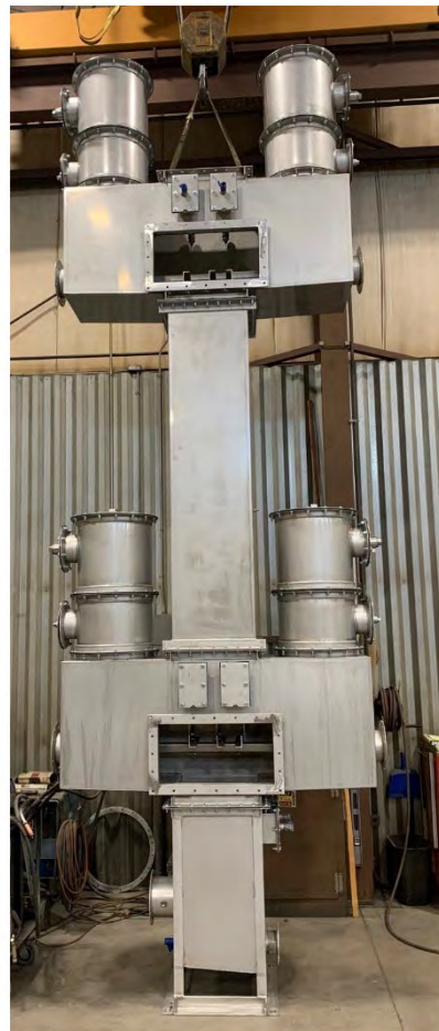
Figure 1. Photo of the pilot-scale WESP.
