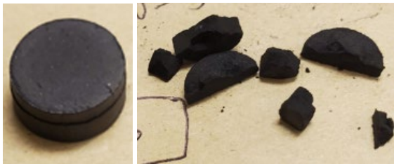
Figure 3: 100wt.% coal sintered at 900°C.
