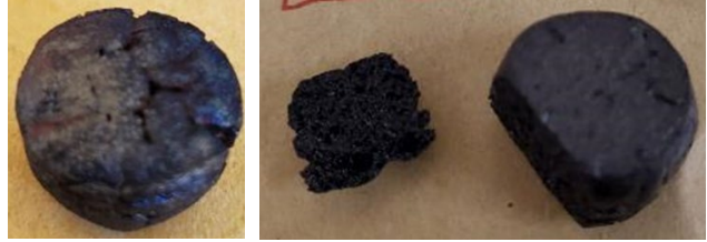
Figure 6: Low strength compacts - coal(10wt.%) - additive (90wt.%) coal sintered at 900°C.
