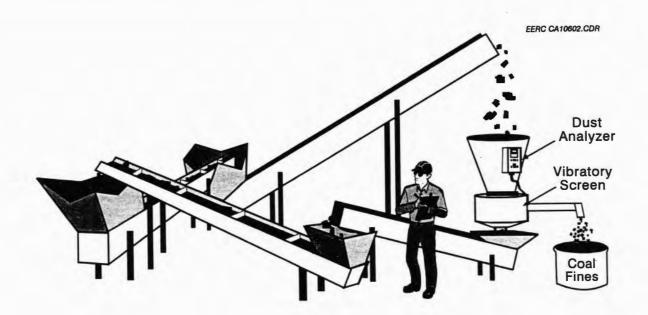
Figure 1. Test loop assembly.
