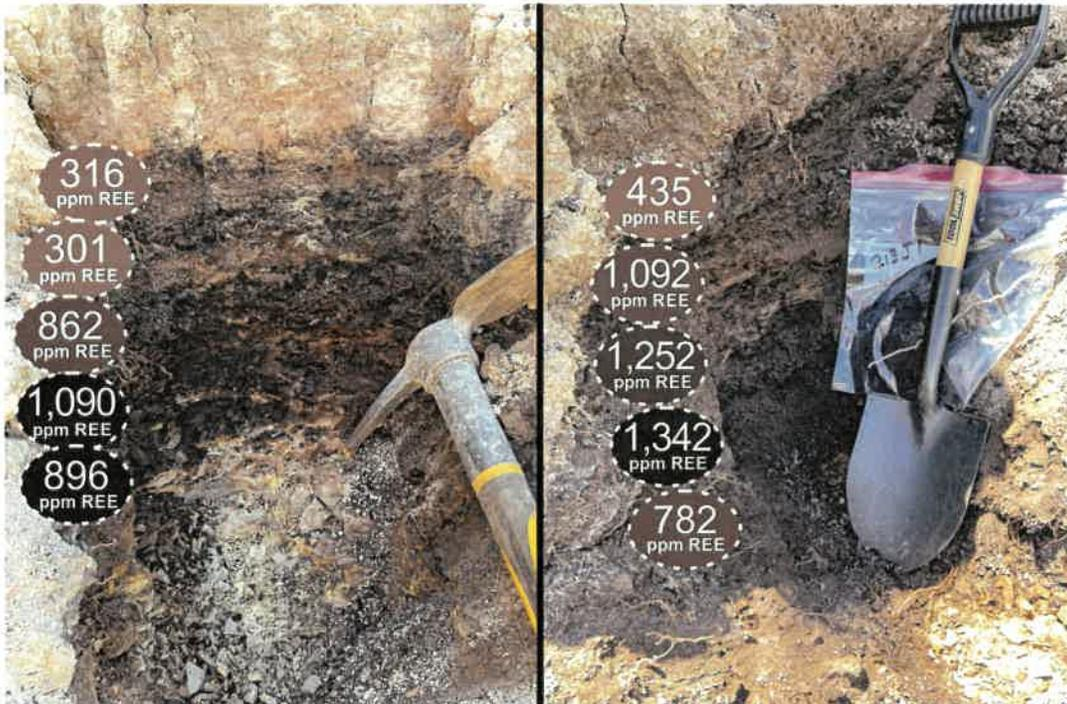
*A thin lignite/carbonaceous bed (15 -22 inches thick) at the base of the Rhame bed in measured sections 210 (left) and 213 (right) located approximately 400 feet apart at Logging Camp Ranch in Slope County. The section 210 coal averages 693 ppm rare earth elements and the section 213 coal averages approximately 980 ppm.*
