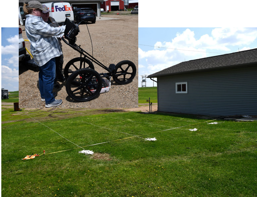
The area north of the garage is gridded for the ground penetrating radar and resistivity surveys. Inset photo: Brittany Brooks and Margaret Patton (background), State Historical Society of North Dakota, ready the three-wheeled ground penetrating radar device for operation.
