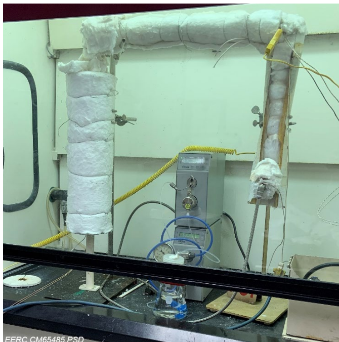
Figure 5. Experimental setup for evaluating the hydrolysis of liquid-phase salts.
