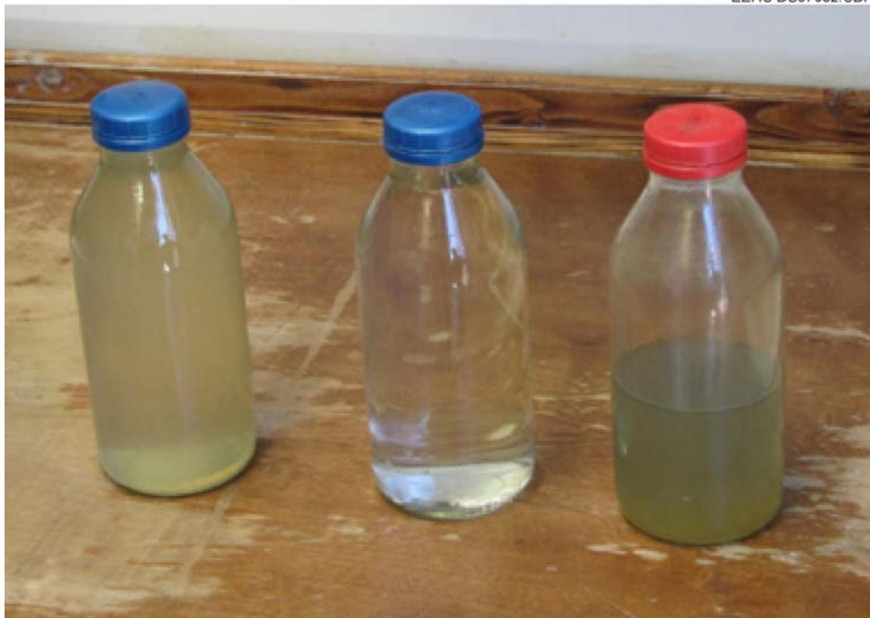
Figure 17. Water samples: frac flowback (left), treated water (center), and MVR concentrate (right).
