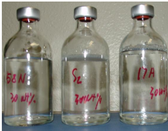
Fig.9 (a) and (b) — Aging at 110°C and 30 %TDS before and after 50 days
