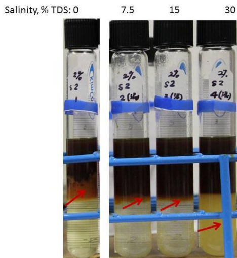
Fig.24a — Phase behavior of S-2 at 23°C
