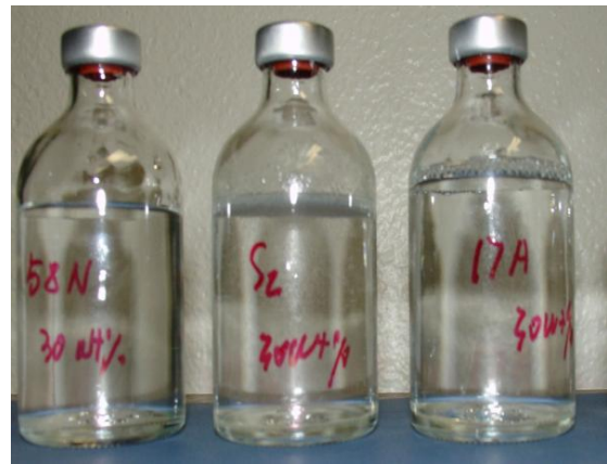
Fig.9 (a) and (b) — Aging at 110°C and 30 %TDS before and after 50 days
