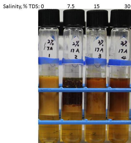
Fig.29a —Phase behavior of 17A at 23°C
