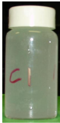
Fig.5 — C-1 alone aging at 23°C
