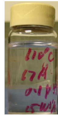
Fig.8 — 17A before and after 0.1% alkaline added aging at 110°C after 7 days
