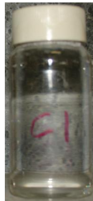
Fig. 6 — C-1 after 30% alcohol added aging for 15 days
