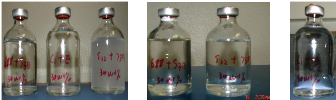
Fig.17 — Co-surfactant aged before and after 50 days and 17 days (right) at 110°C
