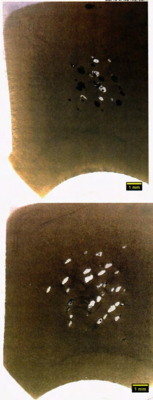
Figure 2. Thin cross sections of single vanes from the green (top) and black (bottom) guides showing extensive but similar rounded porosity.
