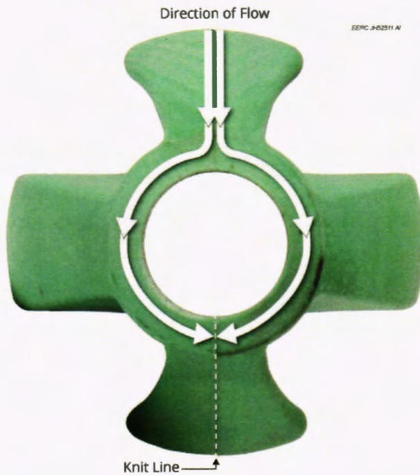
Figure 11. Simplified view of the formation of a knit line during injection molding.
