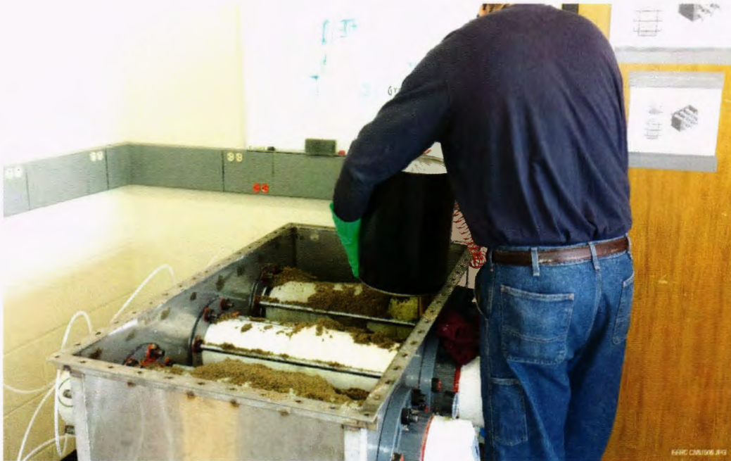
Figure 4. Second 20 gallons of crude oil being added.
