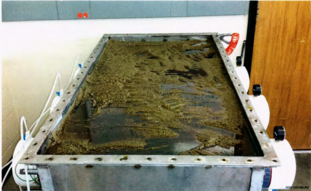
Figure 6. View of the fully saturated sand before the top cover was applied.
