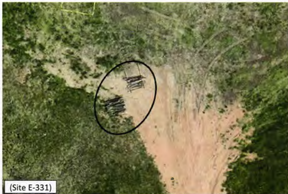
Figure 35: Infrastructure detection in an intermediate restored site (E-331); pipes and debris have been picked-up from the site and stockpiled, but have not yet been removed from the site
