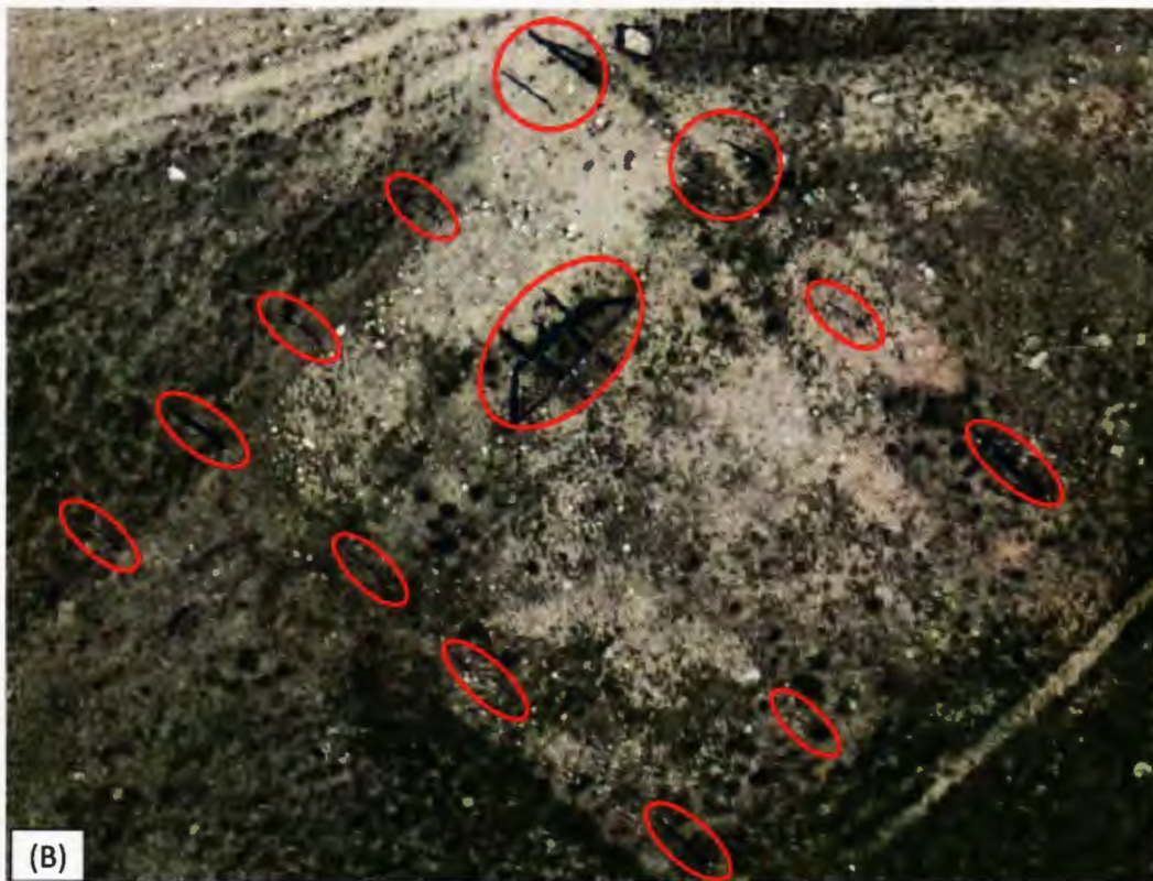
Figure 34B: Visual detection of piping infrastructure of various sizes in RGB imagery at 3-cm resolution are also clearly visible at modest image enlargement (image not maximum zoom).
