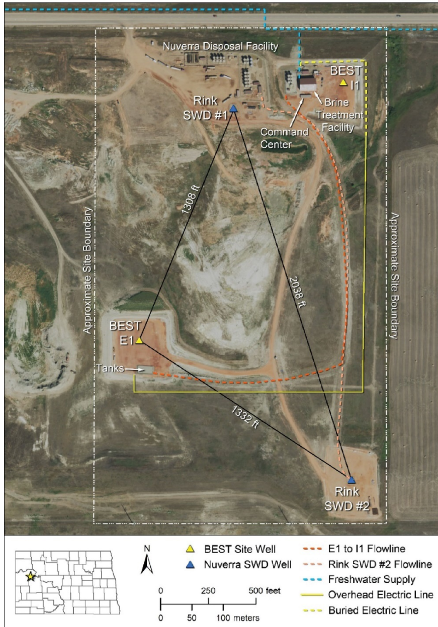
Figure 3-16. BEST project site. Fluid samples were collected from the BEST E1 well to test the efficacy of the GHCR concept at a commercial SWD site.
