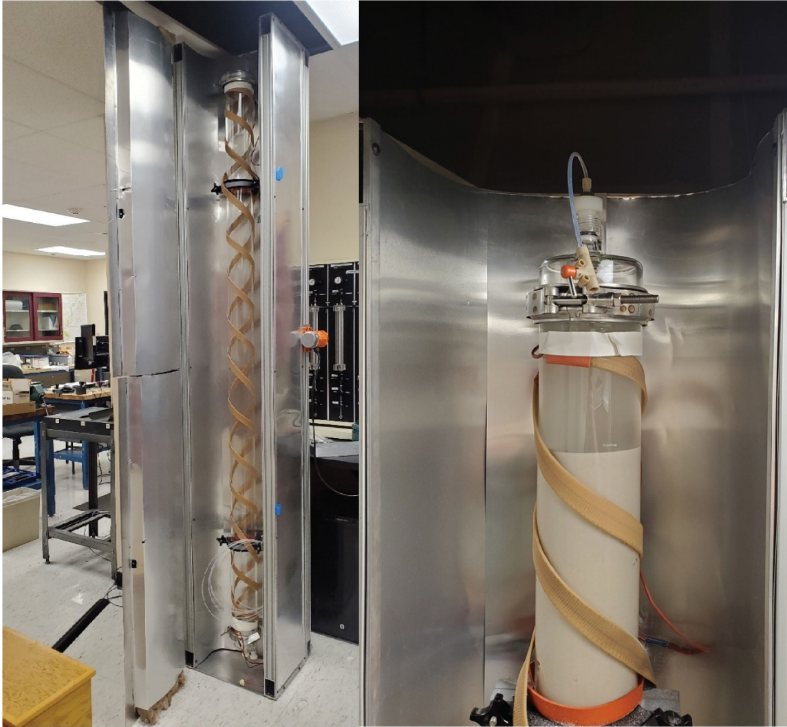
Figure B-1. Left – glass column mounted to insulated aluminum enclosure ready to be filled with sand. Right – column in the last stages of being filled with saturated sand. Glass end cap installed for pulling vacuum.
