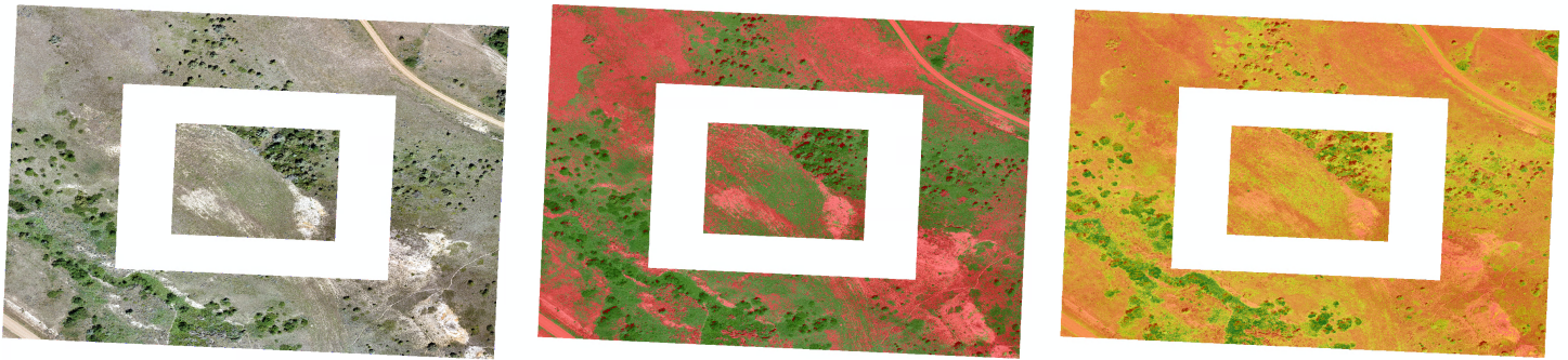
Figure 13. The Blacktail Federal BN_1_25_100MSDCF well location imagery (at left), vegetation classification with vegetation in green and bare soil in red (at center), and vegetation vigor (at right) where green represents higher vegetation vigor or health.
