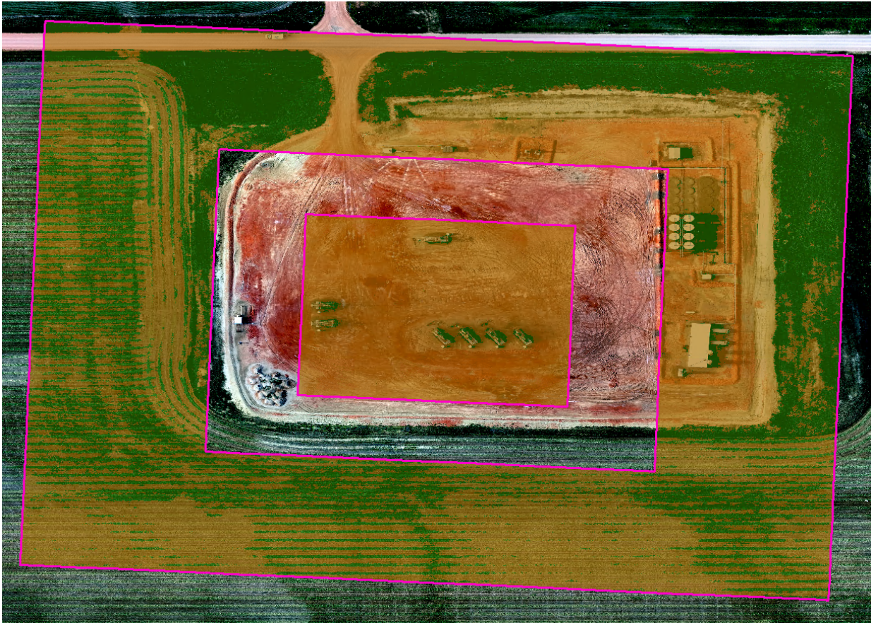
Figure 1. Example of vegetation classification analysis around an operating well pad based on UAV imagery. Green indicates vegetation, and brown indicates bare soil, litter, or gravel. Note that, while effective at classifying vegetation, some structure shadows are erroneously classified as vegetation due to the shadows possessing spectral signatures similar to vegetation spectral signatures.
