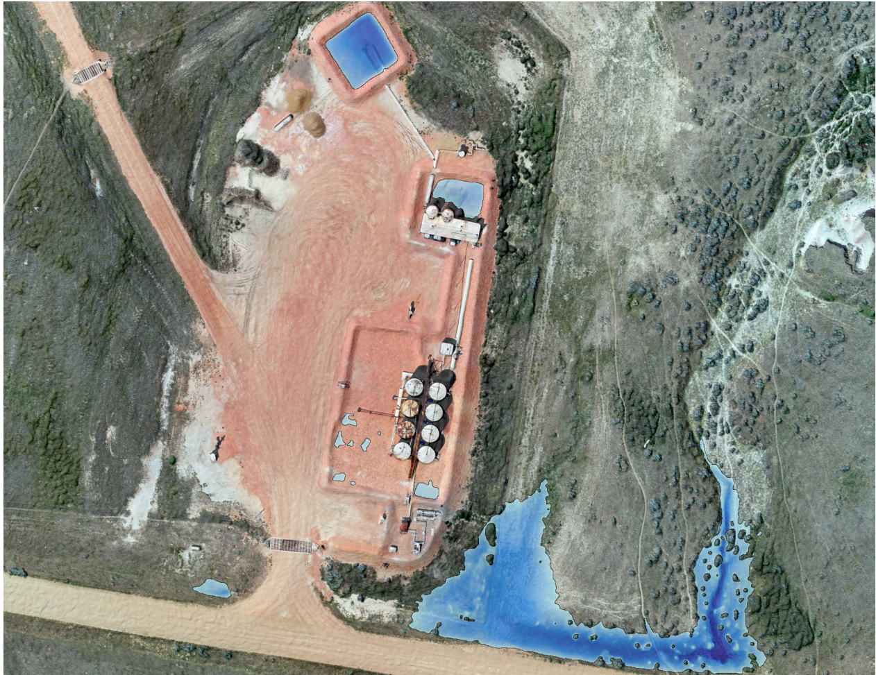
Figure 18. Example showing inundation zones on- and off-pad. On-pad inundation zones occur within the spill containment zones. Off-pad inundation zones depict where water will accumulate following heavy rainfall events. The surface hydrology analytic can be used to assess the effectiveness of stormwater mitigation devices on and around the well pad.
