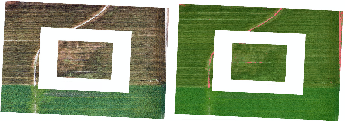
Figure 12. Image at left is the unaltered orthomosaic and image at right is the model output where classified bare soil is red and classified vegetation is green.
