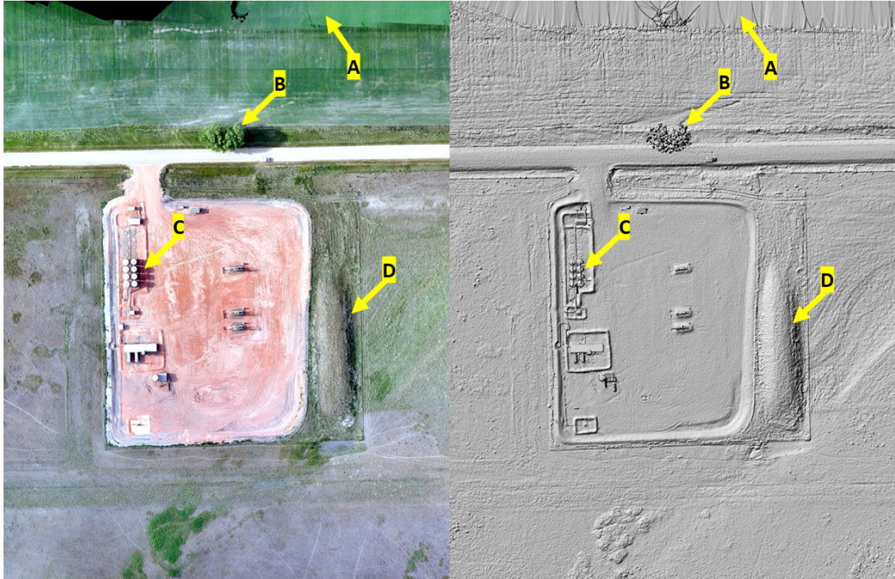
Figure 7. Example of an orthomosaic and associated digital surface model hillshade for a pad with four features highlighted in yellow. Feature A is interpolation noise that is a product of not enough photograph overlap or areas that are very spectrally homogeneous. Feature B is a tree that has higher elevation values than the surrounding terrain, which is useful for calculating tree structure but poses issues when calculating terrain slope or surface hydrology since the tree feature is considered part of the terrain. Feature C is storage tanks on the pad. Notice how infrastructure features have sharp elevation values with homogeneous tops. Feature D is a stockpile for reclamation purposes. This feature can be delineated and total volume calculated with the volumetrics analytic.
