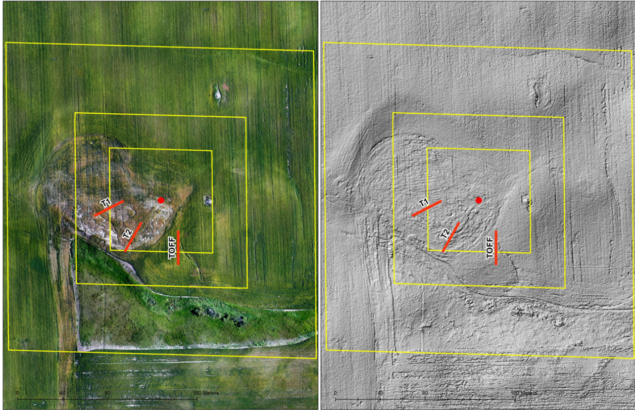
Figure 27. The Christen 24-10 orthomosaic (at left) and digital surface model hillshade (at right) with pad and reference areas considered in the vegetation cover analytic outlined in yellow and in-field vegetation cover transects depicted in red.
