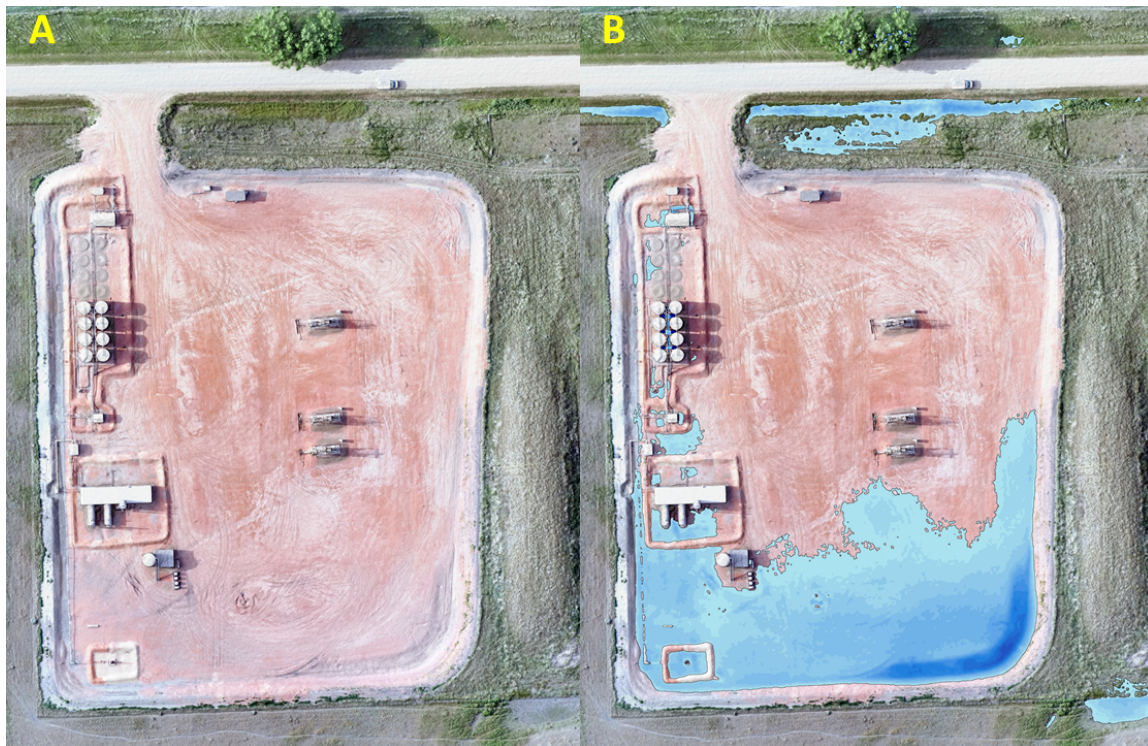
Figure 6. Example of inundation analysis on a functioning pad. Exhibit A is the orthomosaic of the pad, and Exhibit B is the inundation analysis for the pad, with darker blue indicating deeper inundation.
