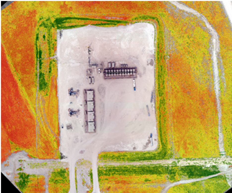
Figure 2. Example of vegetation vigor analysis around an operating well pad based on UAV imagery. Green indicates healthy vegetation (i.e., high levels of chlorophyll), and red and orange colors indicate vegetation that is senescent or has low levels of chlorophyll. This analysis was developed using a modified version of the TGI index that utilizes components of the GLI and NGRI indices.
