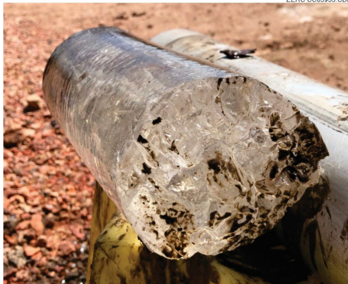
Figure 5-2. Dunham clear crystal salt. Grain size (measured in crosscut) averages 1 in., with minimum and maximum sizes of 0.25 and 2.5 in.
