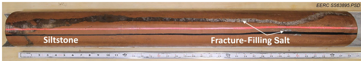
Figure 6-4. Salt-filled fractures in siltstone (Core Run 3, Box 9).
