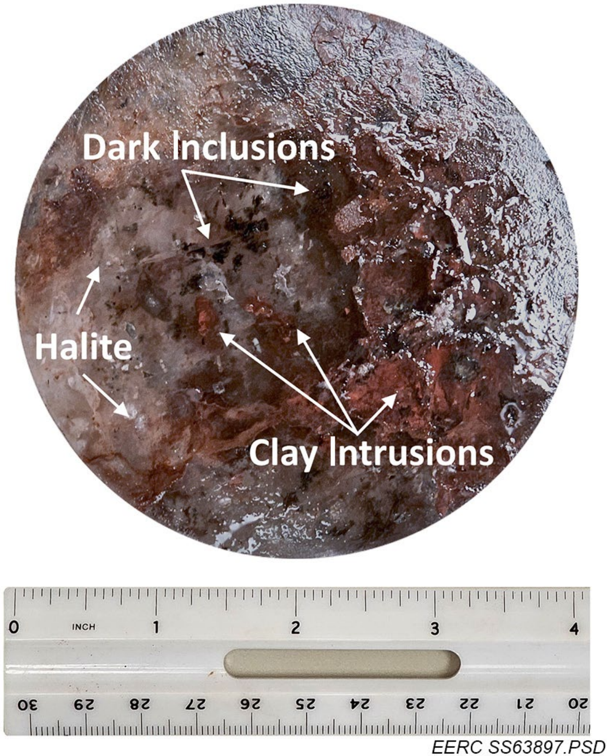
Figure 6-6. Clay intrusions and dark inclusions between halite crystals (7185.80 ft).
