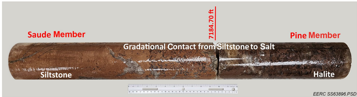
Figure 6-5. Gradational contact into mostly halite (Core Run 3, Box 10 to 11).
