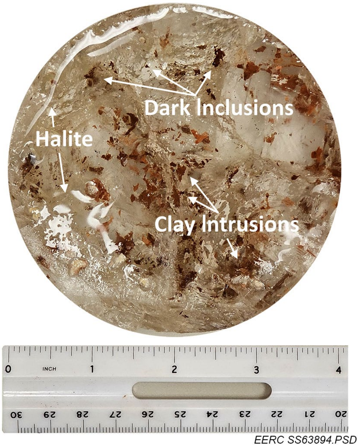
Figure 6-3. Red-brown clay intrusions with small dark inclusions visible (6848.10 ft).
