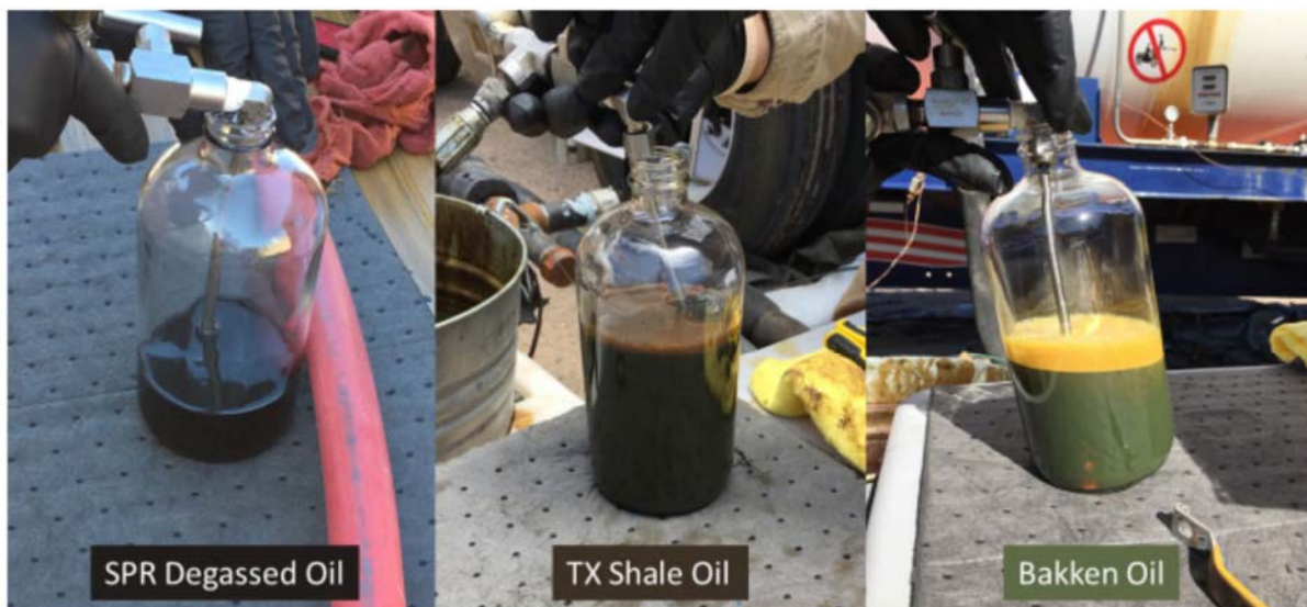
Figure F- 15: Photos of the crude oil samples taken by open bottle sampling method the week of July 16, 2018 (oil temperature 75-80°F, ambient pressure ~11 psia @ ~7,000 ft elevation).
