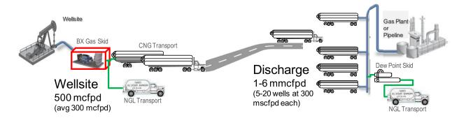
At the discharge point the tube trailers are dropped off and connected to a manifold. The tubes are depressurized and drained through a discharge facility. Gas is sold to a gas gatherer or pipeliner.
