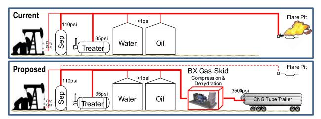
The compressor skid boosts the pressure from 15 psig to 3,500 psig, which enables the tube trailer to carry 210mcf per load. A well making 500 mcfpd would require about 3 loads a day. The gas will be dehydrated to under 0.5 lb/mmcf water content before being transported by CNG tube trailers.
