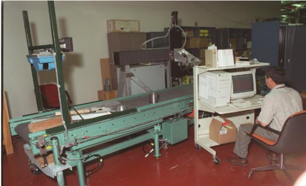
Figure 1 Prototype Conveyor Waste Assay System
