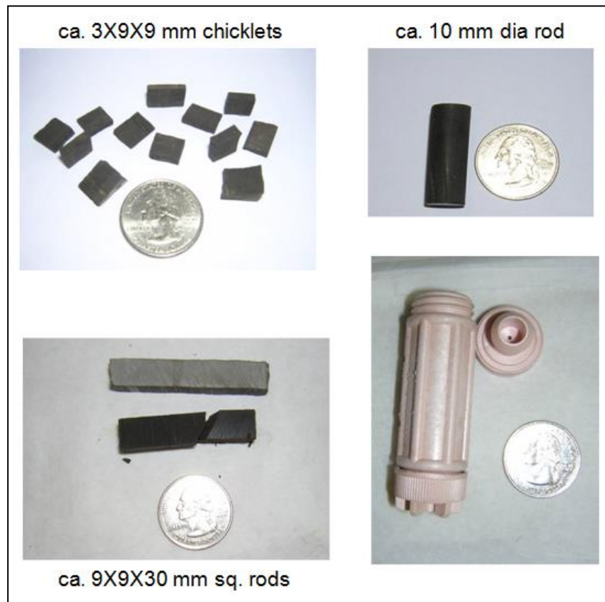
Figure 2. Typical reservoir and source rock samples prepared for CO 2 exposure. Samples are placed in the 10 mL extraction vessel (15 mm i.d. X 57 mm long, lower right), and exposed to CO 2 as described in the text.
