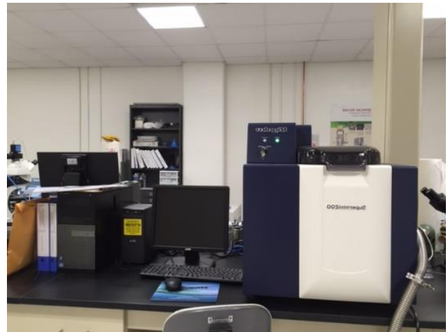
Figure 2: XRF analyzer installed at the UND, Advanced Petroleum Engineering Laboratory (APEL)
