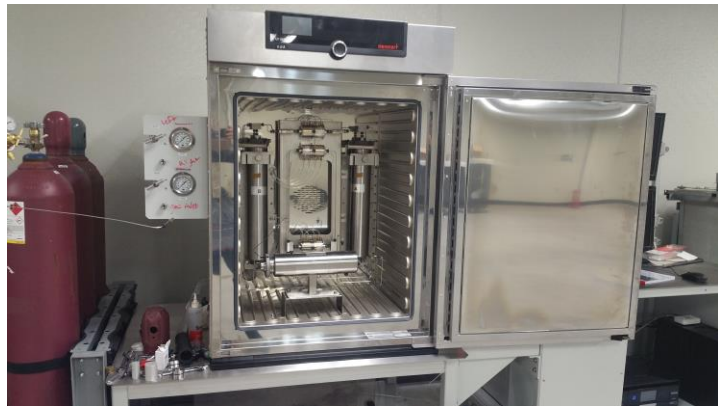
Figure 8: Coreflood tester installed at the UND, Advanced Petroleum Engineering Laboratory (APEL)
