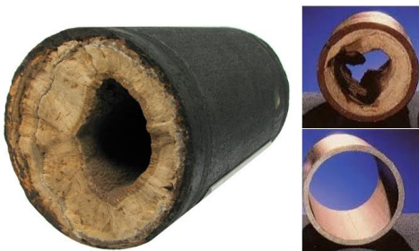
Figure 10. Tubing fouled with calcium-carbonate scale [Courtesy of Schlumberger, 2017]
