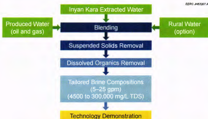
Conceptual extracted water treatment flow diagram.
