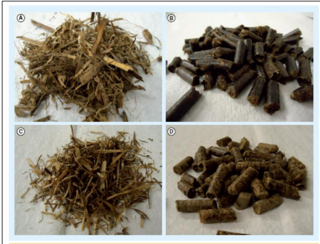
Figure 9. Packed bed Ammonia Fiber Expansion-treated biomass. (A) corn stover, loose; (B) corn stover, pellets; (C) wheat straw, loose; (D) wheat straw, pellets. Pellets are 0.25 inches in diameter. (Campbell et al., 2013)
