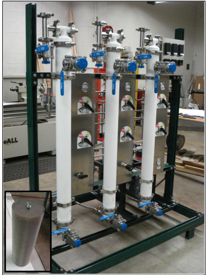
Figure 3. Photo of the packed bed AFEX-3 reactor system. (Campbell et al., 2013)
