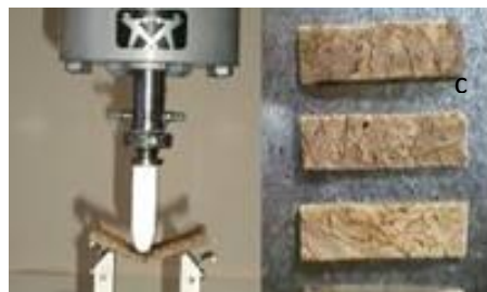
Figure 4. Test jigs a. Three point bending jig b. Bending test c. Internal bond test
