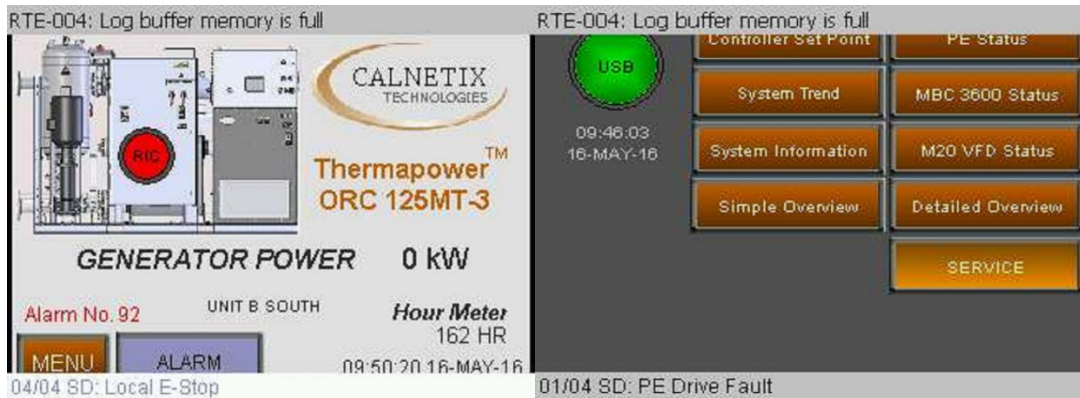
Figure 1.7 Screen shot of the user interface for the system. As a remote site, UND was able to view the primary data, but did not have the ability to access any of the control screens. The screen shots show the system producing 115 kW of electricity.
