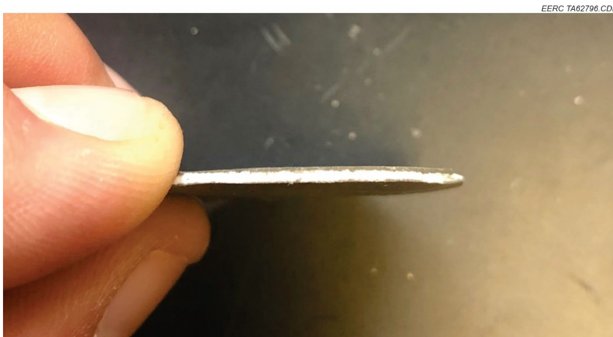
Figure 16. C-PEE-based MEA fabricated via simultaneous three-layer heat-treating process.
