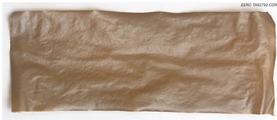
Figure 10. Film-cast PEM comprising 75% CUP–25% PBI.
