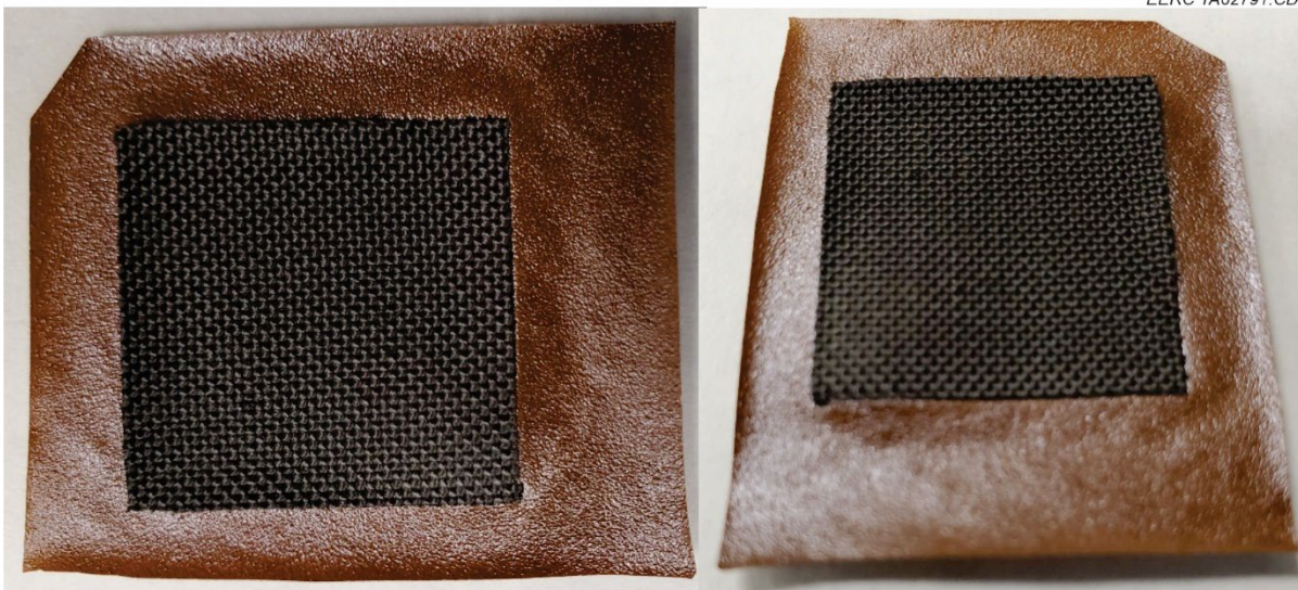
Figure 11. MEA comprising film-cast C-PEE membrane, platinum anode, and ruthenium cathode.
