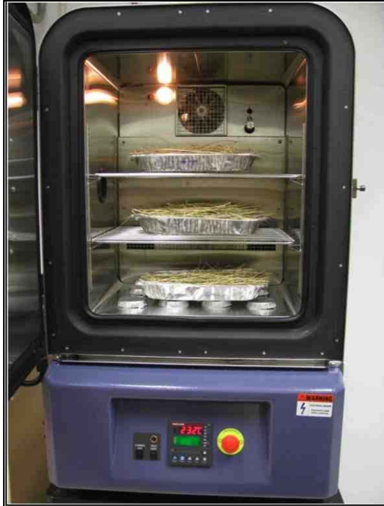
Fig. 12. Environmental control chamber showing samples loaded for hydration or storage characteristics determination
