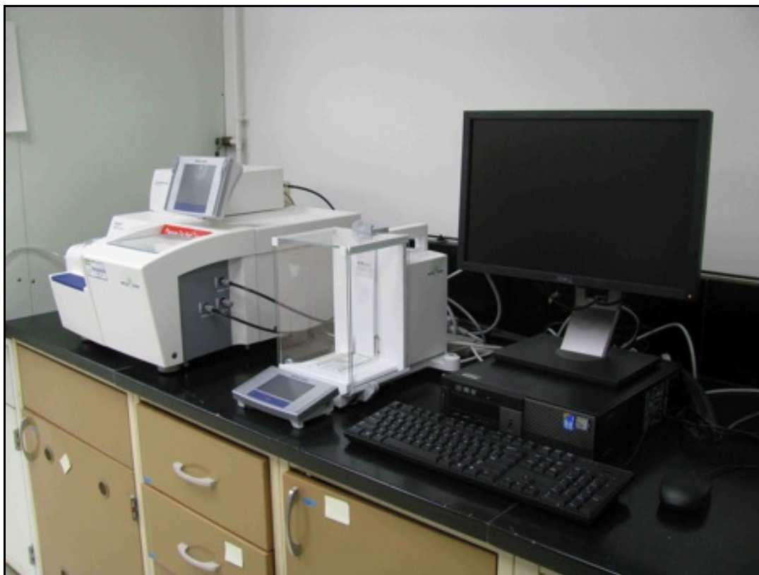
Fig. 3. Thermal analyzer - installed with analytical balance and computer controls
