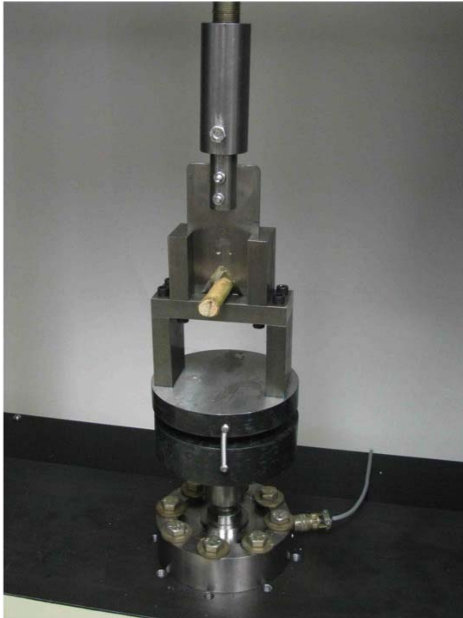
Fig. A7-46. Figure showing indigenously developed and fabricated (Figs. 9 and 10) modified Warner-Bratzler device being used to measure the cutting strength and energy of biomass stems (e.g. corn stalk). The load cell is at the bottom fixed to the bed of UTM and knife is moved down by the crosshead in compression mode. Load cell is loaded through compressing platens.
