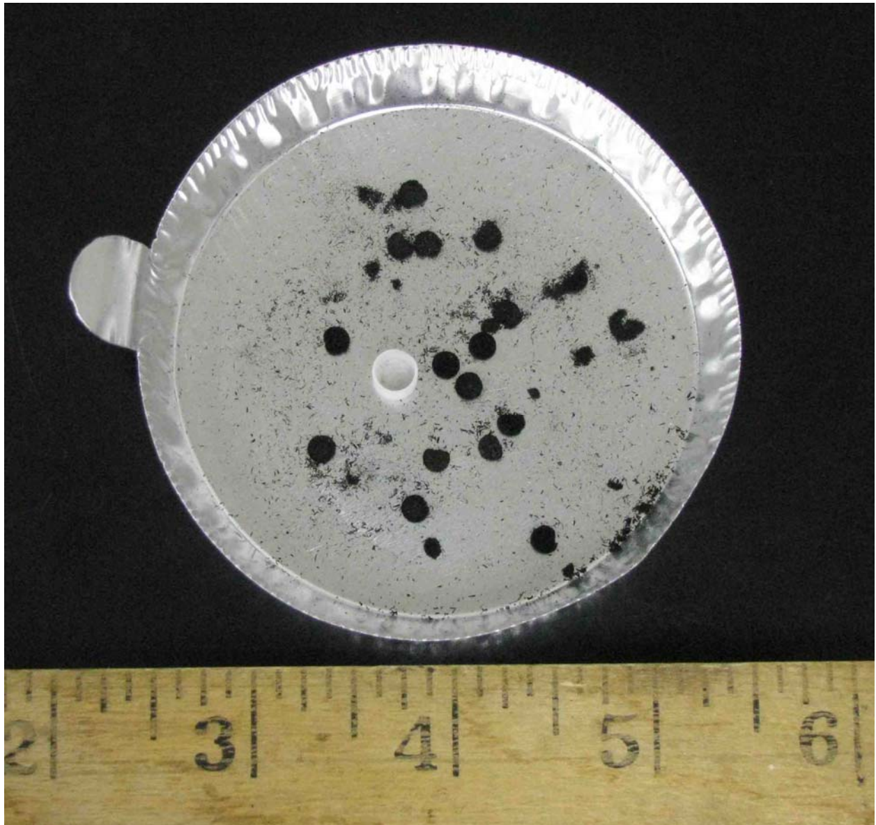
Fig. A7-2. Picture showing alumina sample holder and pyrolyzed ground switchgrass when nitrogen was used as purge gas. Note that in inert environment such as nitrogen only charring occurs and carbonaceous material remains; however, with air (presence of oxygen) only white ash remains
