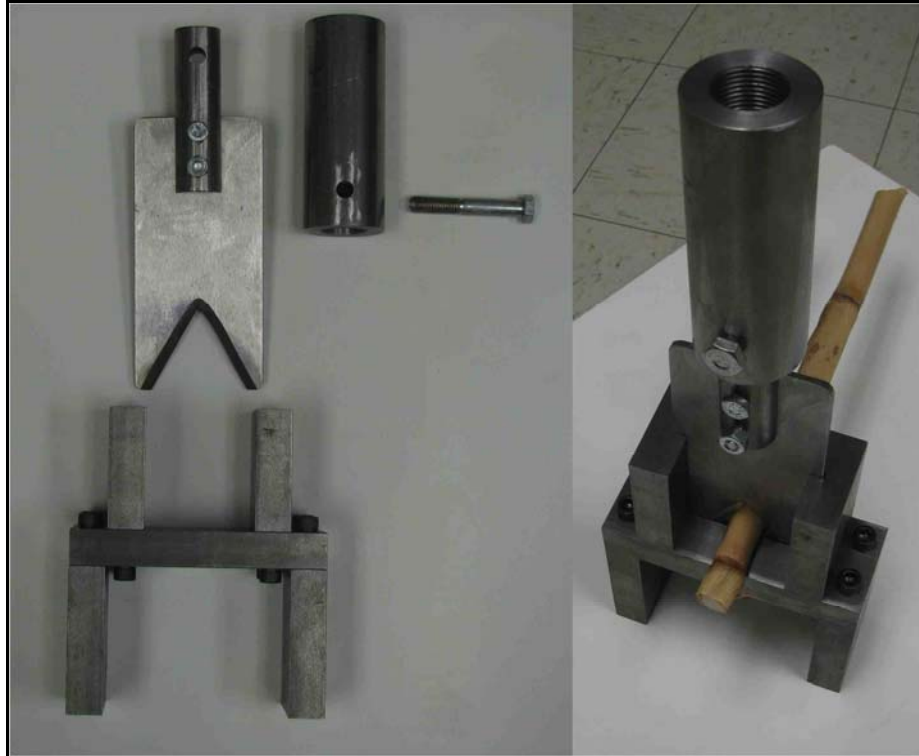
Fig. 10. Components of the indigenously designed modified Warner-Bratzler cutting device for cutting strength determination for biomass; Right – assembly of components illustrating cutting of corn stalks
