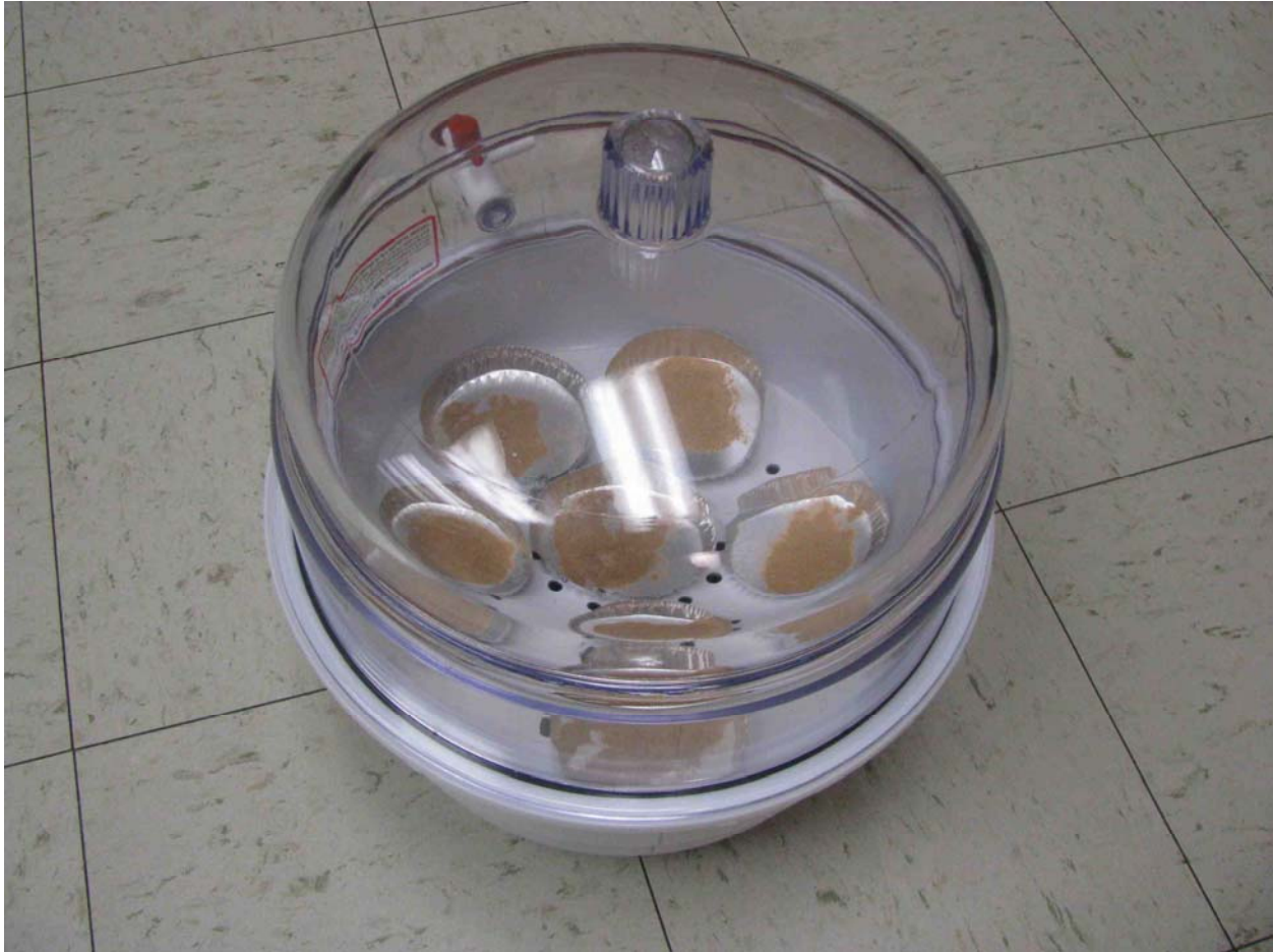
Fig. A5-1. Picture showing ground switchgrass biomass on aluminum dishes being held in desiccator for cooling after the oven drying procedure to obtain the bone dry mass in moisture content determination. The moisture content of the samples used in the study varied from 4.2% to 7.4% wet basis.
