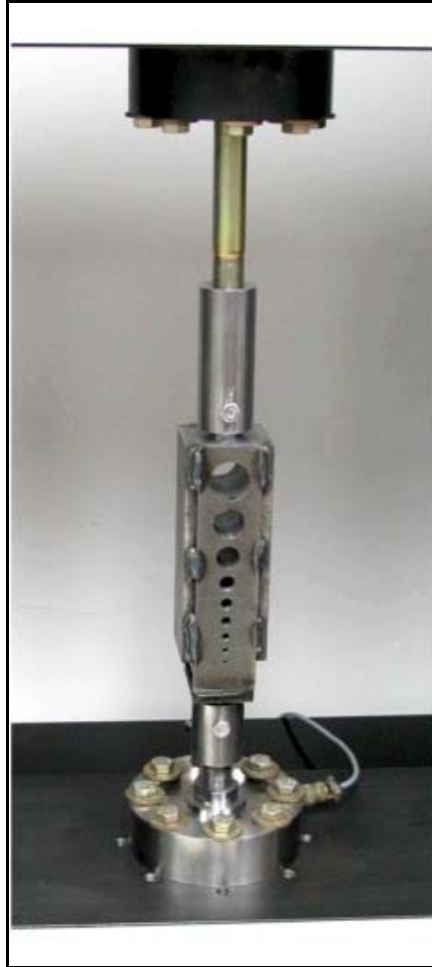
Fig. 7. Indigenously designed and fabricated double-shear device attachment for shear strength determination of biomass
