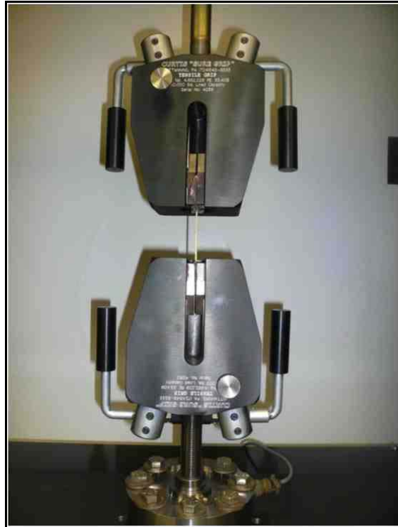
Fig. 8. Commercial tensile grips (Curtis “Sure Grip”) attachment used in the tensile strength determination of biomass
