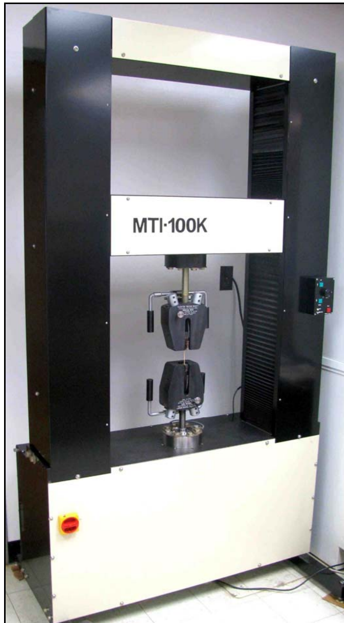
Fig. 5. Universal testing machine with tensile grips for tensile strength testing for biomass
