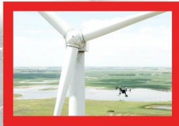
BLADE INSPECTION / ICING MODEL
