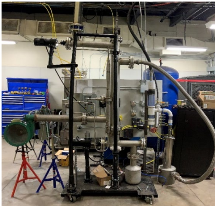
Figure 3. Image of UND's Bench Sandwich Gasifier
