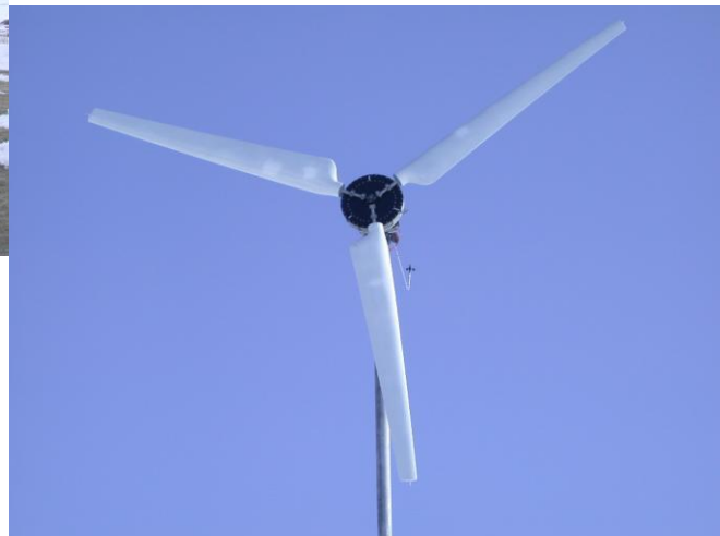
The first Proto-type flying. Note long conduit sticking out front with the anemometer on it!
