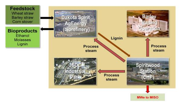
The Spiritwood Expansion Model shows how the biorefinery fits into the Spiritwood industrial site as feedstock intake and bioproducts producer as well as a CHP steam partner and lignin (solid fuel) provider.
